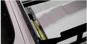
DOUBLE CAB - Remove the rubber molding on the roof of the truck. Make sure the rear mount is sitting right next to the edge trim.
