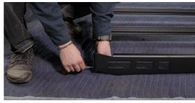
**3.** If you are installing a light bar, remove the bolts to one side of the cross bar and slide in 4 T nuts (2 per side). Then you can install the light bar brackets to the crossbar and install your light bar.
