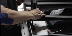
**10.** Use the long M6 bolts with washers to secure the mounts to the roof. Hand thread the bolts and then use a 5/32 allen to loosely tighten the bolts. Be careful when tightening the mounting bolts into the nutserts. You do not want to cross thread the bolts.
