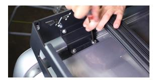
12. Reinstall the factory rubber molding. You will have to cut it since the mounts are in the way. Use 3M tape to secure it back into place. The last step is to add the edge trim to the fairings and adjust them. We recommend adjusting them down against the roof for added support, to eliminate any flex at high speeds.
