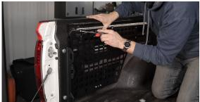
**5.** Center the bottom bracket then tighten it. Using a 5/16" drill bit, drill two holes through the opening of the lower bracket and into the side of the bed. You will need someone to help you secure two bolts through the holes from the under side of the truck (inside the fender area).
