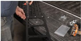
3. Connect the two brackets. Place the triangle bracket on top of the other bracket and connect them with two button head bolts. Using two more button head bolts, connect the bracket to the bottom of the panel.
