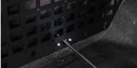
**6.** There are many different mounting options. Below we will show you how to install the high lift mount. Put a carriage bolt through the built-in slot and secure it with a 1/2" washer and nut. Tighten the bolts down with an 11/16" wrench. Then use a wing nut to secure the high lift jack.
