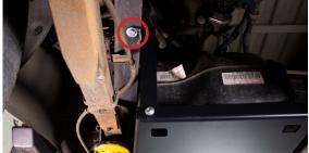
3. Once the 2 holes are drilled, the skid can be loosely installed using the hex head hardware in the 2 locations where you drilled, and the button head hardware everywhere else. Ensure all hardware is loosely installed before tightening any bolts.
