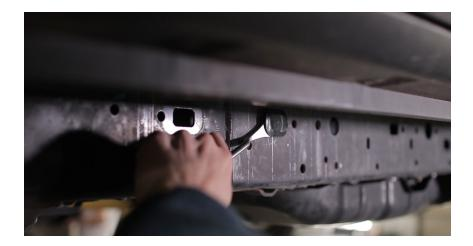
5. Now we will bolt the slider on. Use a jack or have a friend help you hold the slider in place. Take the large washer and stack the medium size washer on top of it followed by a flange nut. This will go on the inside of the frame rail. Use a 1/2" bolt with a washer and thread it into the flange nut on the inside of the frame rail.
