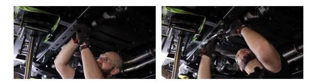
**7.** Go back and tighen the bolts along the frame. Reconnect the brake line along with the gas tank cover and the plastic cover that sits inside the frame.
