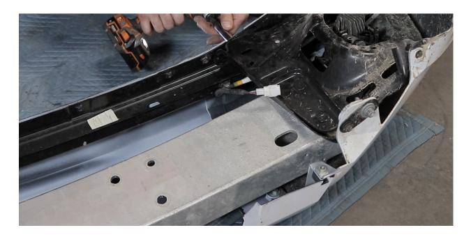
**6.** Using a 14mm socket, remove the 3 bolts on each side that connect the light bracket to the cross bar.
