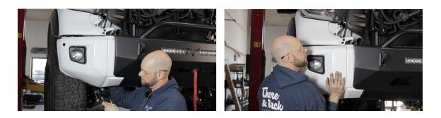
Next, loosen the bolt under the fog light to move the bumper inward or outward, to create an even gap between the Victory & factory bumpers.
