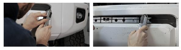
**3.** Unplug your fog lights and proximity sensors. This will be essential when you remove the crash bar. Using a 17mm socket, remove the 6 nuts holding the crash bar in place. After you remove the crash bar, use a 14mm socket to remove the nuts as shown in the picture below. There will be 4 nuts to remove on each side and we will use them later to install the blitz bumper. Once the nuts are removed, throw away the frame horns.
