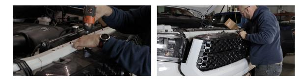
2. Using a body saw, cut along the groove as shown in the pictures below. After you remove the bumper you can go back and clean up the edges of the trim.
