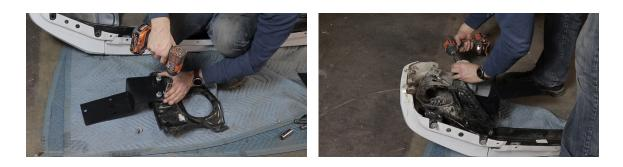
**8.** Before we can install the bumper we need to move the cooler back. Start by removing the 12mm bolt on the right side and slowly bend the bar back.
