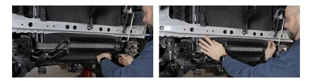
Use a bracket that we supply and place it over the 12mm bolt hole. Use the button head bolt we supply to connect our bracket to the factory bracket on the cooler.
