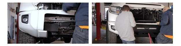
Next you will loosely reinstall the 14mm nuts we removed earlier. The easiest way to install these is to reach around the side. Then reinstall the bolts on the bottom of the bumper with a 17mm socket. Once the bottom bolts are tight, you can tighten the 14mm bolts behind the bumper.
