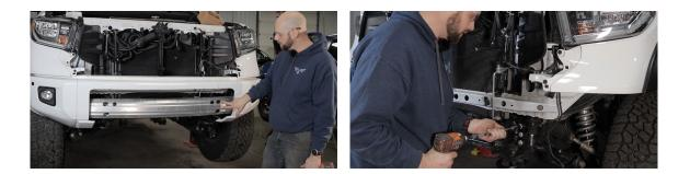
**4.** Next we will remove the tow points. Using a 17mm socket, remove 2 bolts per tow point.
