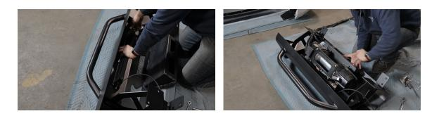
**10.** Install the blitz bumper. Make sure you align the bolt holes with the preexisting bolts. Next, have a friend help you lift the blitz bumper onto the pre-existing bolts.
