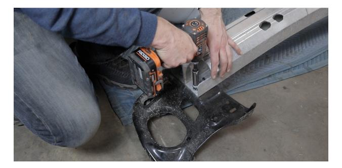
7. Using a 14mm socket, attach the new bracket to the light bracket with the nuts we removed earlier. Then reattach the light bracket to the bumper using the 4 bolts (per side) we removed earlier.
