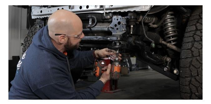
**5.** Using a 12mm socket, remove the 4 bolts on each side holding the light bracket in place.
