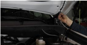
2. Use a 12mm socket to tighten down the bolts. Make sure the hinge is in the same place as it was before we loosened the bolts. Run your wire through the inside hole and secure it with a zip tie.
